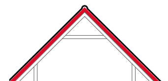
Insulation above the rafters
