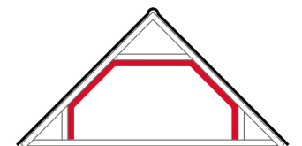
Insulation between the rafters
